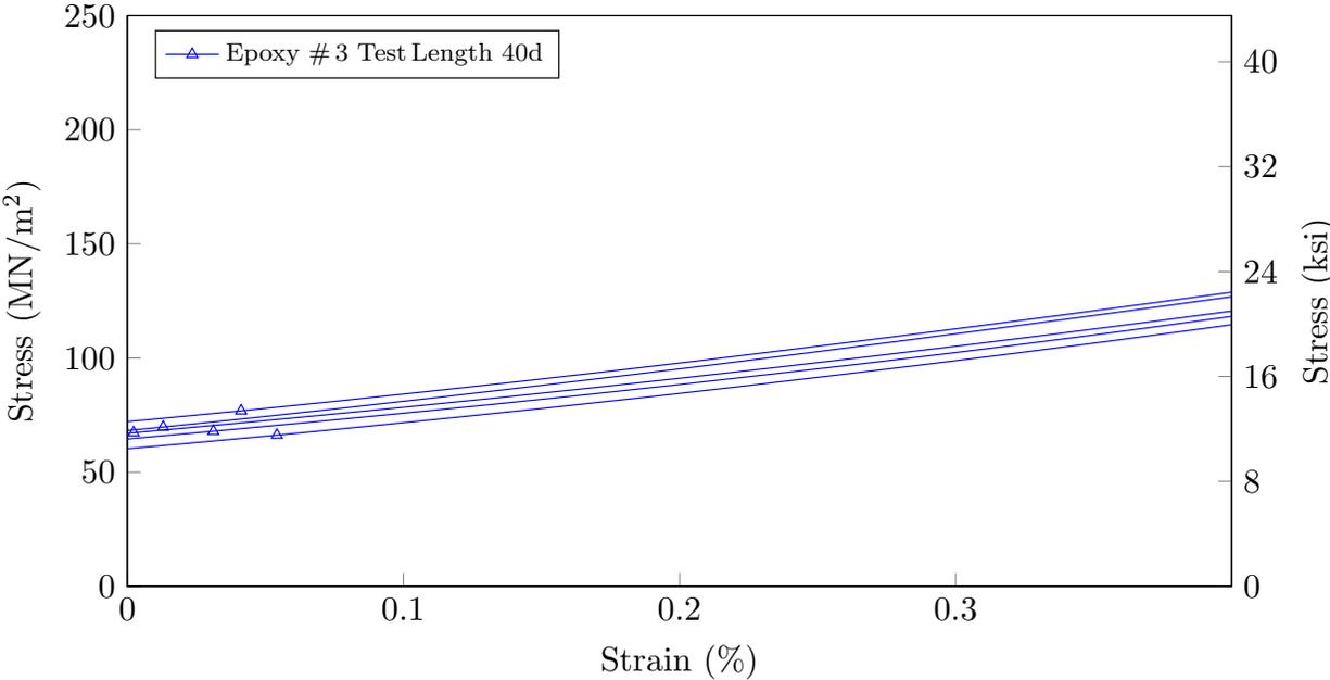
Figure 7.3: Tensile stress vs Strain behavior of RockRebar<sup>®</sup> Lot 1 Epoxy rebar size 3
