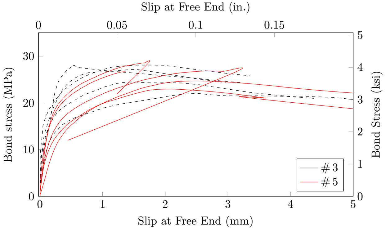
Figure 8.4: Free end slip behavior of the tested RockRebar<sup>®</sup> #3 and #5
