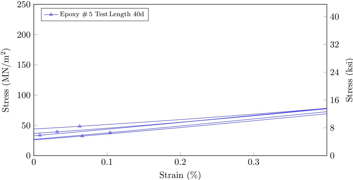
Figure 7.4: Tensile stress vs Strain behavior of RockRebar<sup>®</sup> Lot 1 Epoxy rebar size 5
