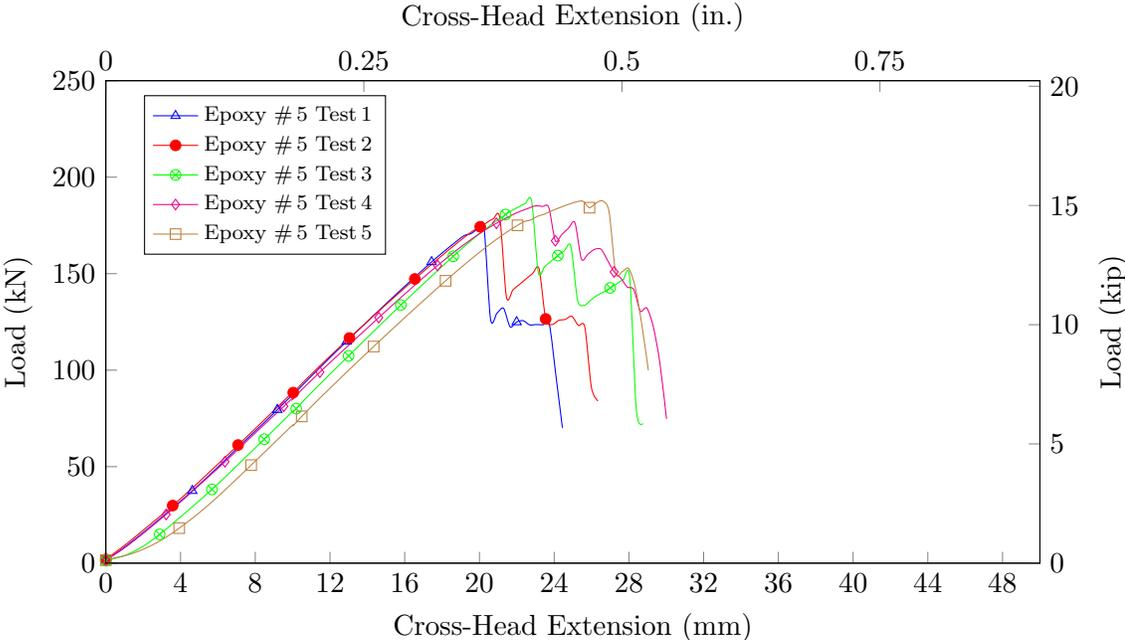
Figure 7.2: Tensile test results for RockRebar<sup>®</sup> #5 with Epoxy resin
