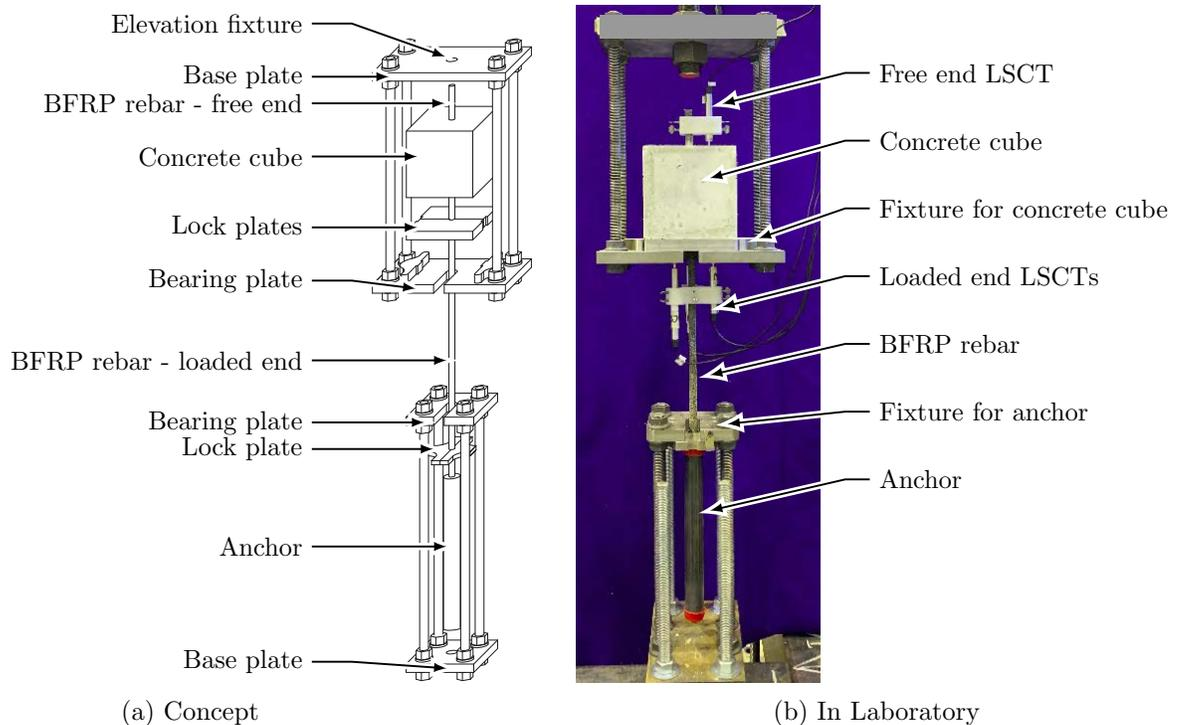
Figure 8.1: Experimental Setup
