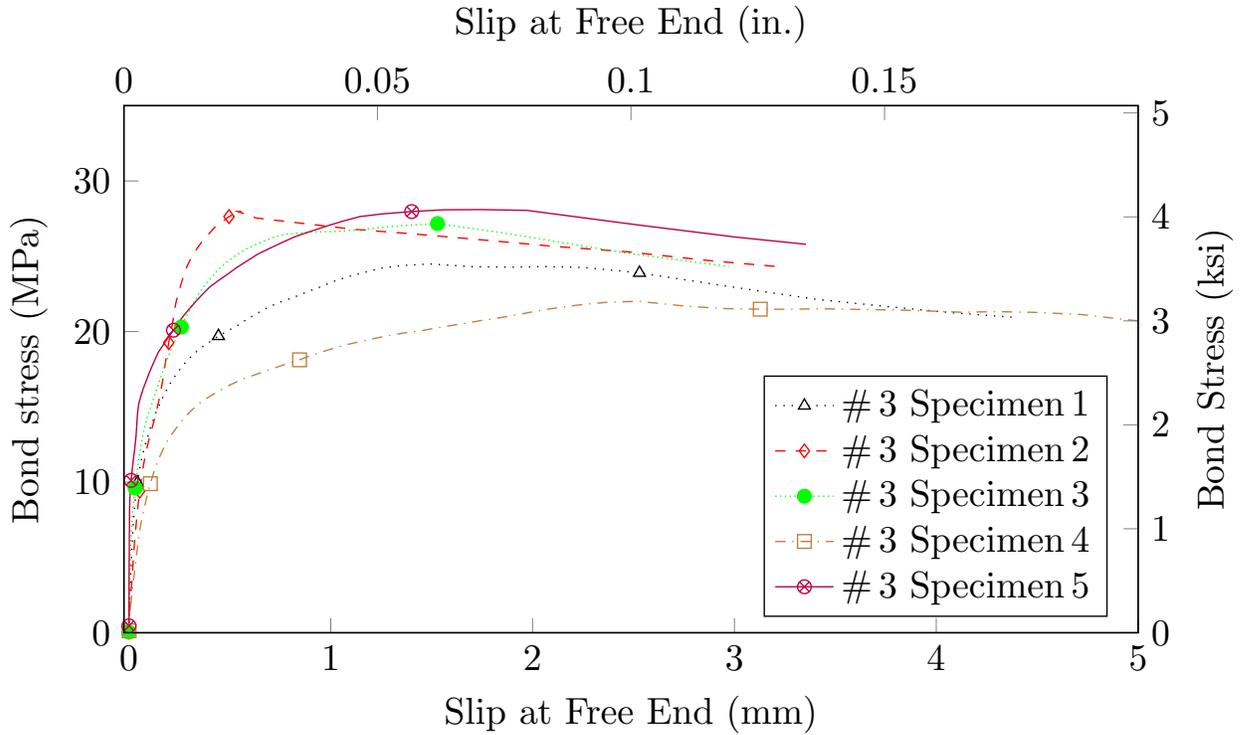
Figure 8.2: Free end slip behavior of the tested RockRebar<sup>®</sup> # 3
