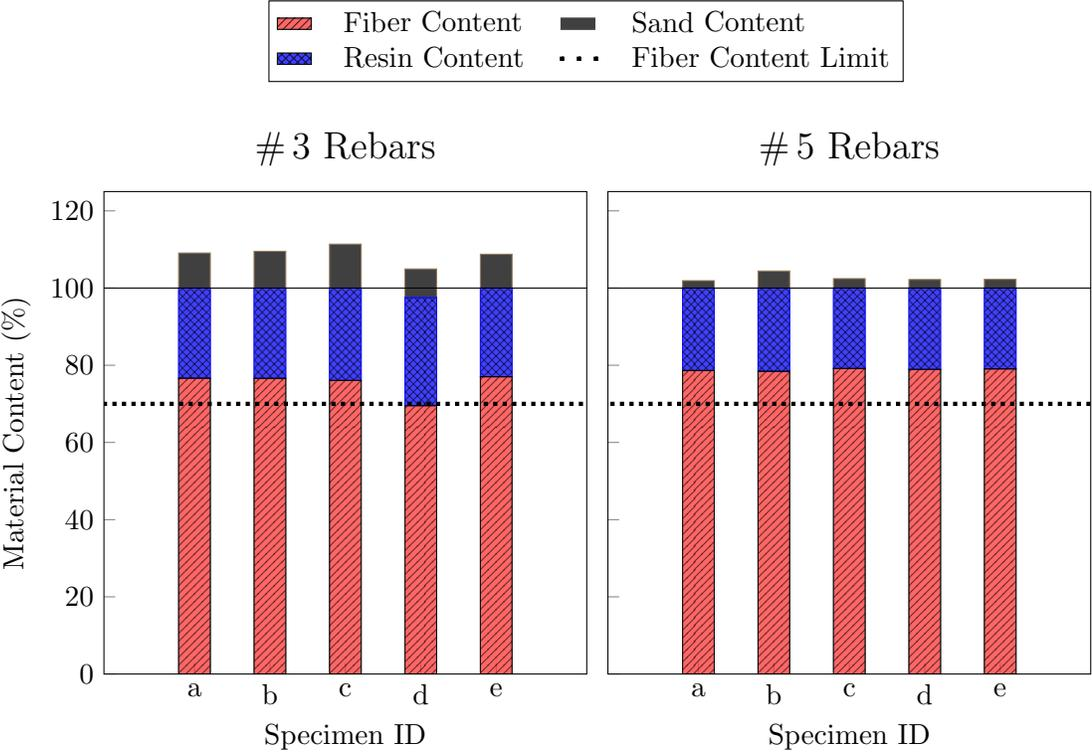
Figure 3.1: Fiber content results of RockRebar<sup>®</sup> with epoxy resin
