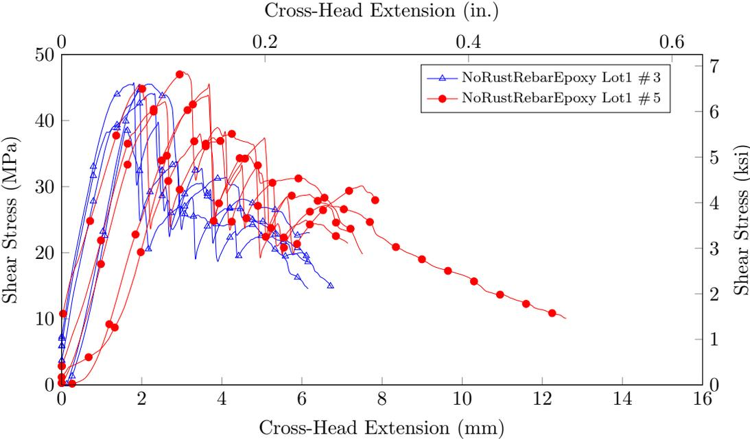
Figure 6.2: Horizontal shear stress vs. extension results for RockRebar<sup>®</sup> Lot 1 #3, and #5 rebar with Epoxy resin
