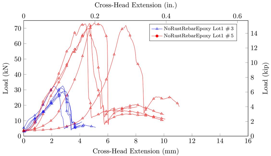
Figure 5.1: Transverse shear test extension vs. load results for RockRebar<sup>®</sup> Lot 1 #3, and #5 rebar with Epoxy resin
