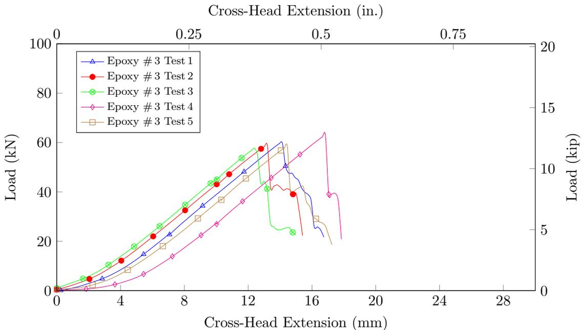
Figure 7.1: Tensile test results for RockRebar<sup>®</sup> #3 with Epoxy resin
