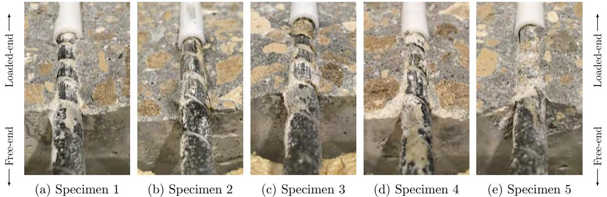
Figure 8.5: Overview rebar surface after testing RockRebar<sup>®</sup> #3
