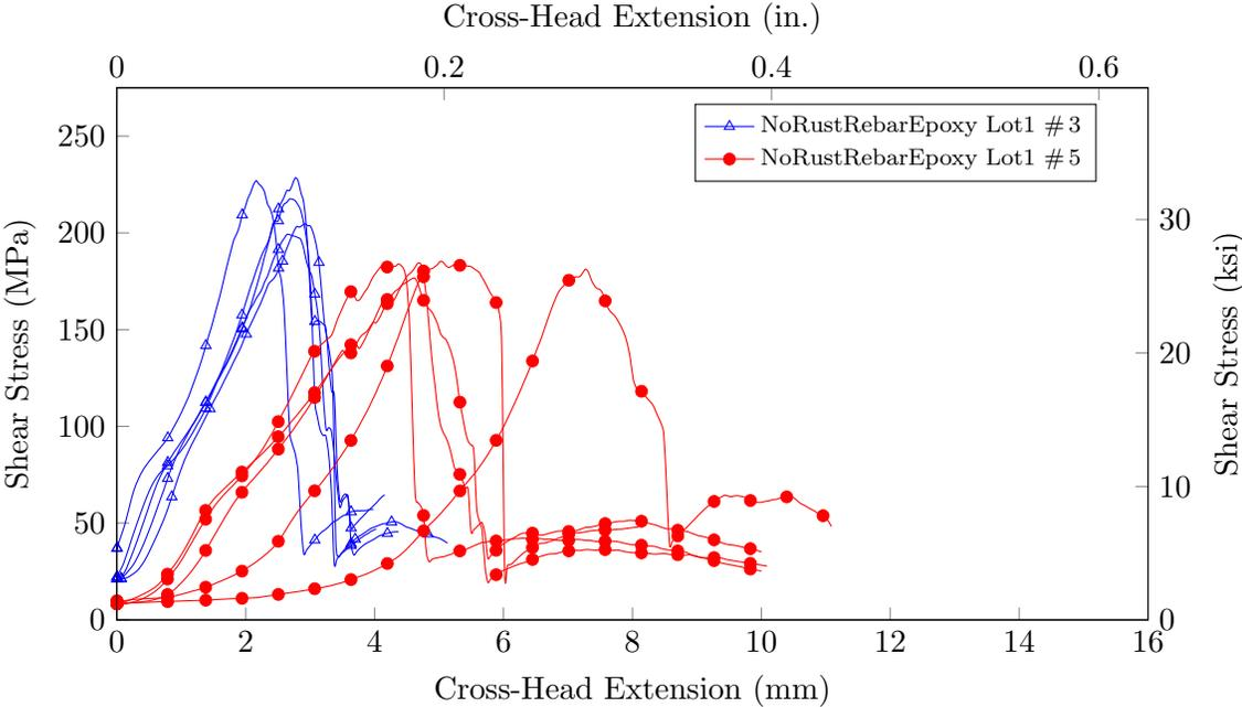
Figure 5.2: Transverse shear stress vs. extension results for RockRebar<sup>®</sup> Lot 1 #3, and #5 rebar with Epoxy resin
