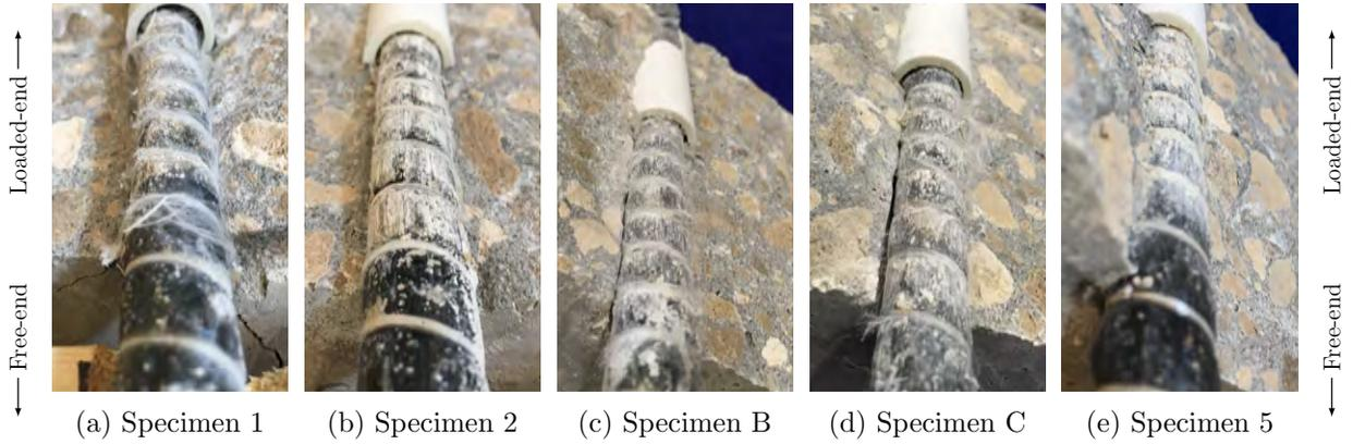
Figure 8.6: Overview rebar surface after testing RockRebar<sup>®</sup> # 5
