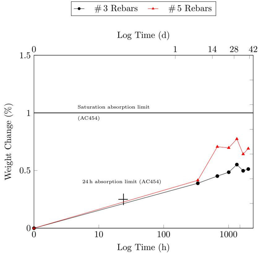
Figure 4.1: Moisture Absorption results of RockRebar<sup>®</sup> with epoxy resin
