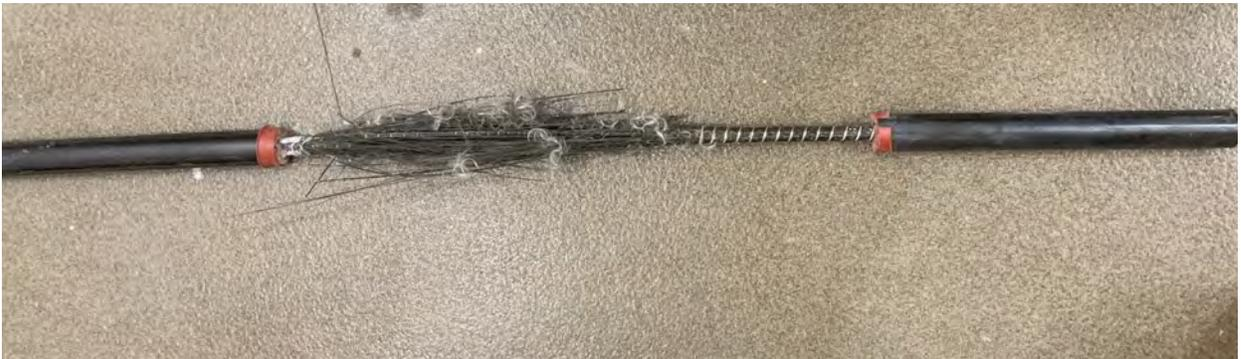
Figure 7.6: RockRebar<sup>®</sup> # 5, final failure pattern after tensile test
