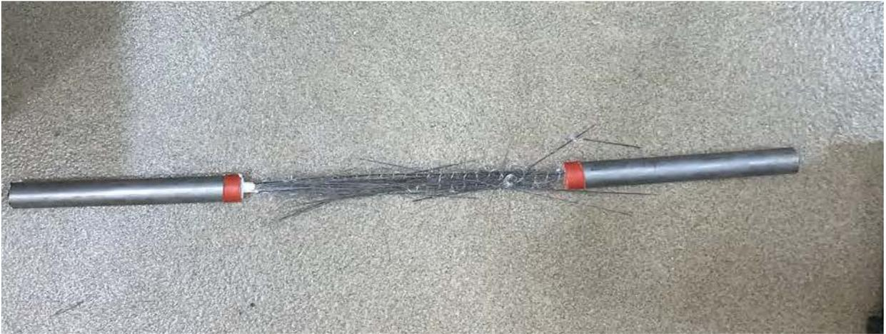
Figure 7.5: RockRebar<sup>®</sup> # 3, final failure pattern after tensile test
