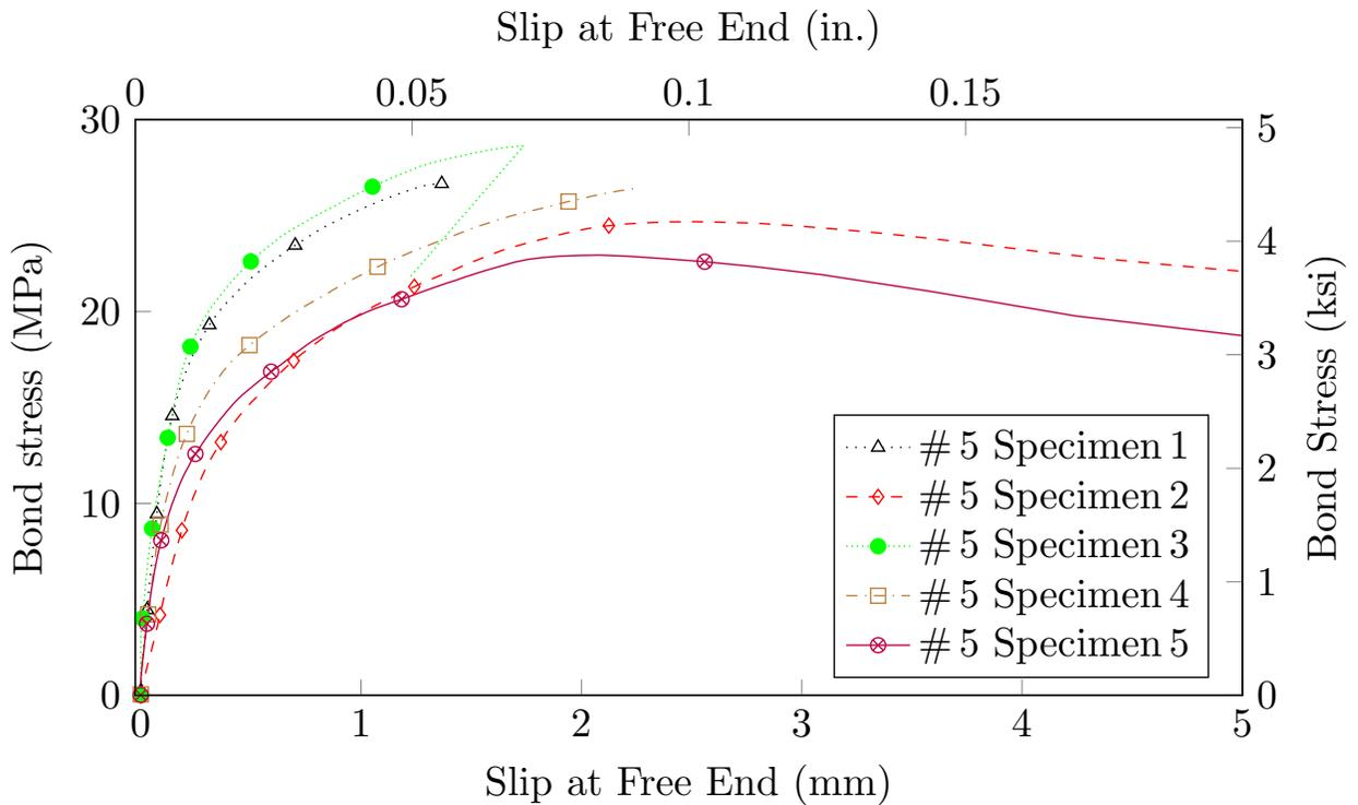
Figure 8.3: Free end slip behavior of the tested RockRebar<sup>®</sup> # 5
