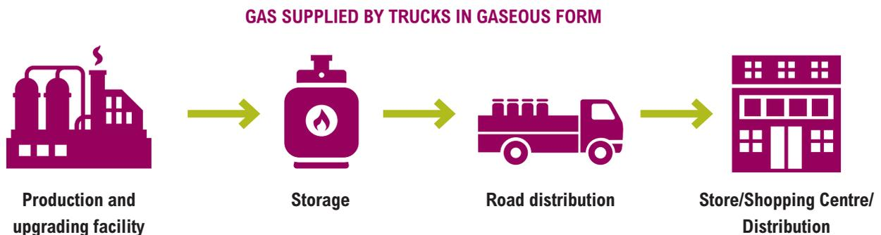
When transported by trucks, biomethane is usually carried or stored in high-pressure cylinders in a range from 200 bar to 250 bar. This option is more energy and cost intensive due to additional operations added to the value chain. This process is more commonly used for long distance transport, such as by heavy duty vehicles or maritime transport.<sup>52</sup>
