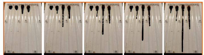
Figure 4: Results of the inclined channel test (Example with four lanes. Start / 20 / 40 / 60 / 100 seconds.)
