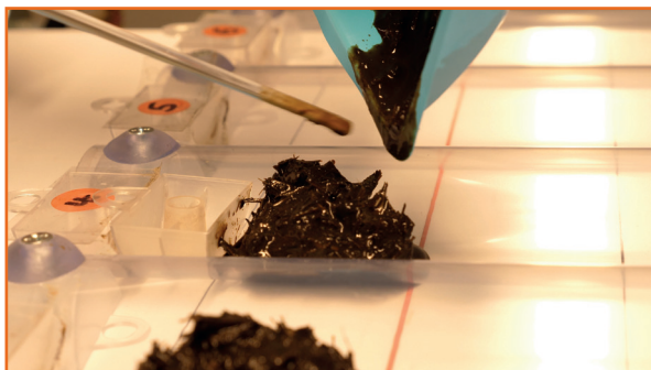
Figure 5: The inclined channel test system (Setup, sample application, in action)
