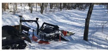
The Ginzugroomer has "teeth" that can chew up old icy snow to recondition it and then set a new track. The new setup also allows the tracksetter to be lifted up to leave a flat packed surface useful in areas with too little snow to set a track and also on steeper grades where not having a track is safer for controlled descent. By packing the trails
