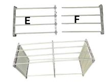
Align the bars on **PART F** with the holes on PART E. Insert by pushing one bar in at a time. Place the holes on the bottom of the Connects on top of the bar tips. Insert one at a time. Push down on the Connects to seat them.
