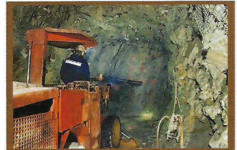
Miners advance the face of the 5-6 level decline, 10' at a time, day and night.
