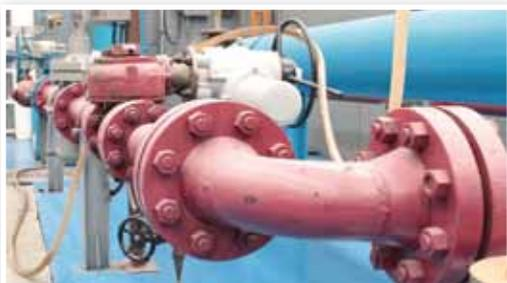
**Test Loop.** A complete Laboratory Test loop exists for design validation of WALWORTH products. The test is performed at maximum design pressure, advances the valves from 3000 to 5000 cycles, and requires more than four months to complete.
