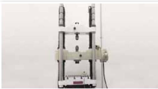
**Tensile Test Equipment.** We use this equipment to verify the mechanical properties of materials used for manufacturing. WALWORTH tests samples on a random basis even though we receive MTRs from our suppliers and foundries.
