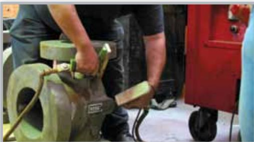
**Magnetic Particle Test.** On a random basis for standard products or when a Customer requests MT Certification, WALWORTH has Magnetic Particle Test Equipment to perform on ferromagnetic materials.
