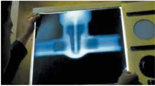
**X-Ray Examination Equipment.** WALWORTH has its own Ir-92 source in-house for the radiographic examination (RT) of castings from 0.100" up to 2 1/2" wall thickness to verify the soundness of the casting raw material.
