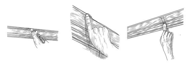
5. Seal joints and gaps with caulking or drywall mud.
