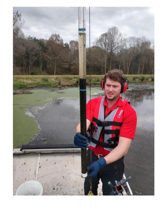
(Click on to see video.) The Sludge was to thick to go into the Lagoon Core Sampler
