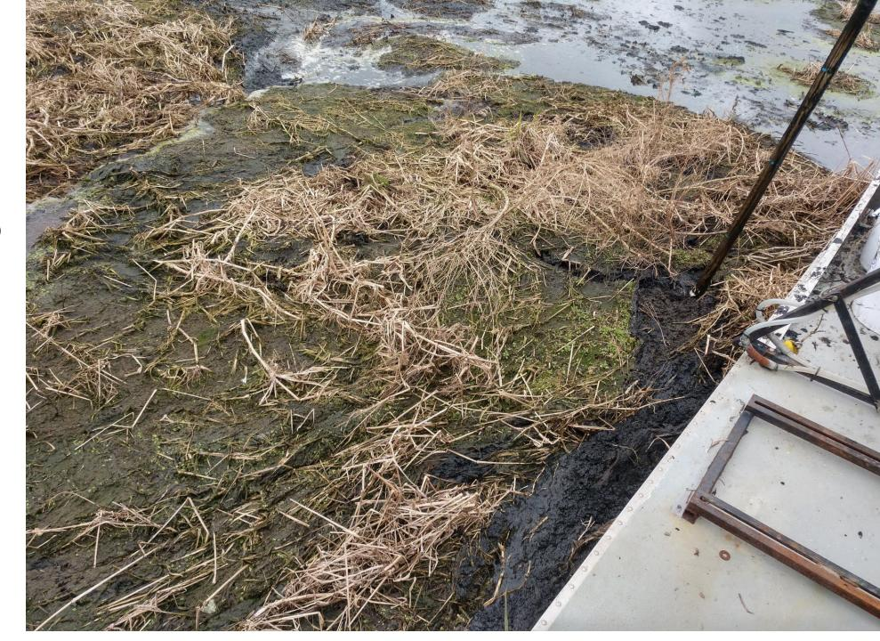
The average depth of this lagoon before the foot of water added, was 5 feet. We were unable to get a full core sample due to the compacted sludge. (See the Video on the next slide.)
