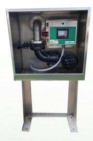
**Fill System for Fuel Tanks.** The Proven Controls Remote Fill is designed for the safe filling of fuel tanks. The system is designed to accept fuel from delivery trucks, safely transfer fuel to the fuel tank and capture fuel leaks in the enclosure. Standard enclosures include tank adapters, manual isolation valves, and check valves.
