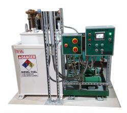
**Day Tank Design.** Standard Day Tanks come in UL142 Rupture Basin, UL142 Double Wall, and UL2085 fire rated versions. Standard components include, but are not limited to suction tubes with foot valves, drop tubes, emergency vent(s), and a primary tank atmospheric vent. Proven Controls day tanks come preassembled with options for flange connections in lieu of threaded connections. All day tanks are designed to meet JHA/ local regulations or site specifications.
