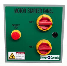
The Motor Starter Panel is designed to start/stop fuel transfer pumps for emergency power applications. The Motor Starter Panel is customized to provide required operating functions for individual or multiple pumps, depending on site specifications or requirements. Standard enclosures are NEMA 3R, 4, 12. Voltage components based on pump voltage requirements.
