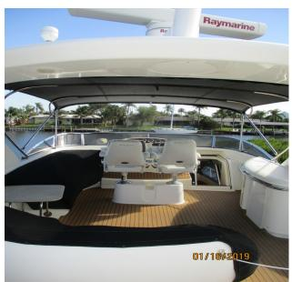
Cored FRP, molded Flybridge. The superstructure mold appeared securely attached to the deckhouse/cabin mold and in sound cosmetic condition No voids or soft spots were noted.
