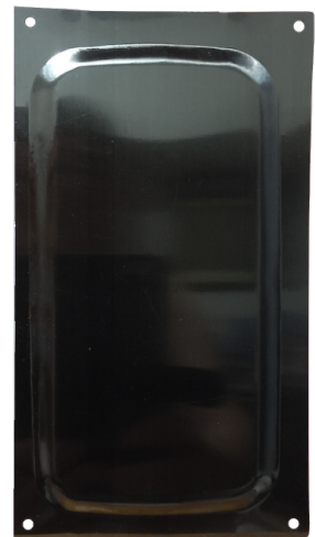
Four edges and four diameter holes by single time punch
