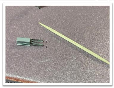
Your hole should be large enough to insert the legs and conduit adjacent. In the photo below I used a clean toothpick to ensure the conduit wires did not become detached or not go into the hole. Once satisfied with fit, secure with a small amount of white glue.
