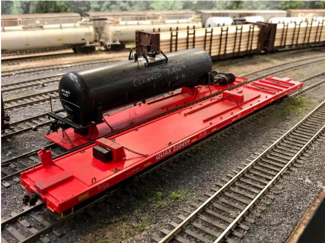
Railcar with empty deck in place and empty deck sitting beside.
