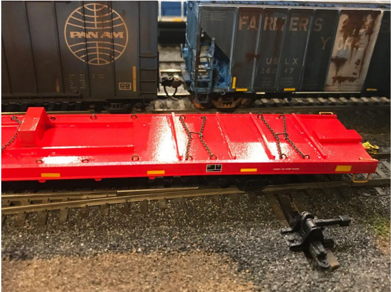
Wheel garden area of railcar with securement chains. The car can not only carry the wrecked railcar but also both sets of trucks.
