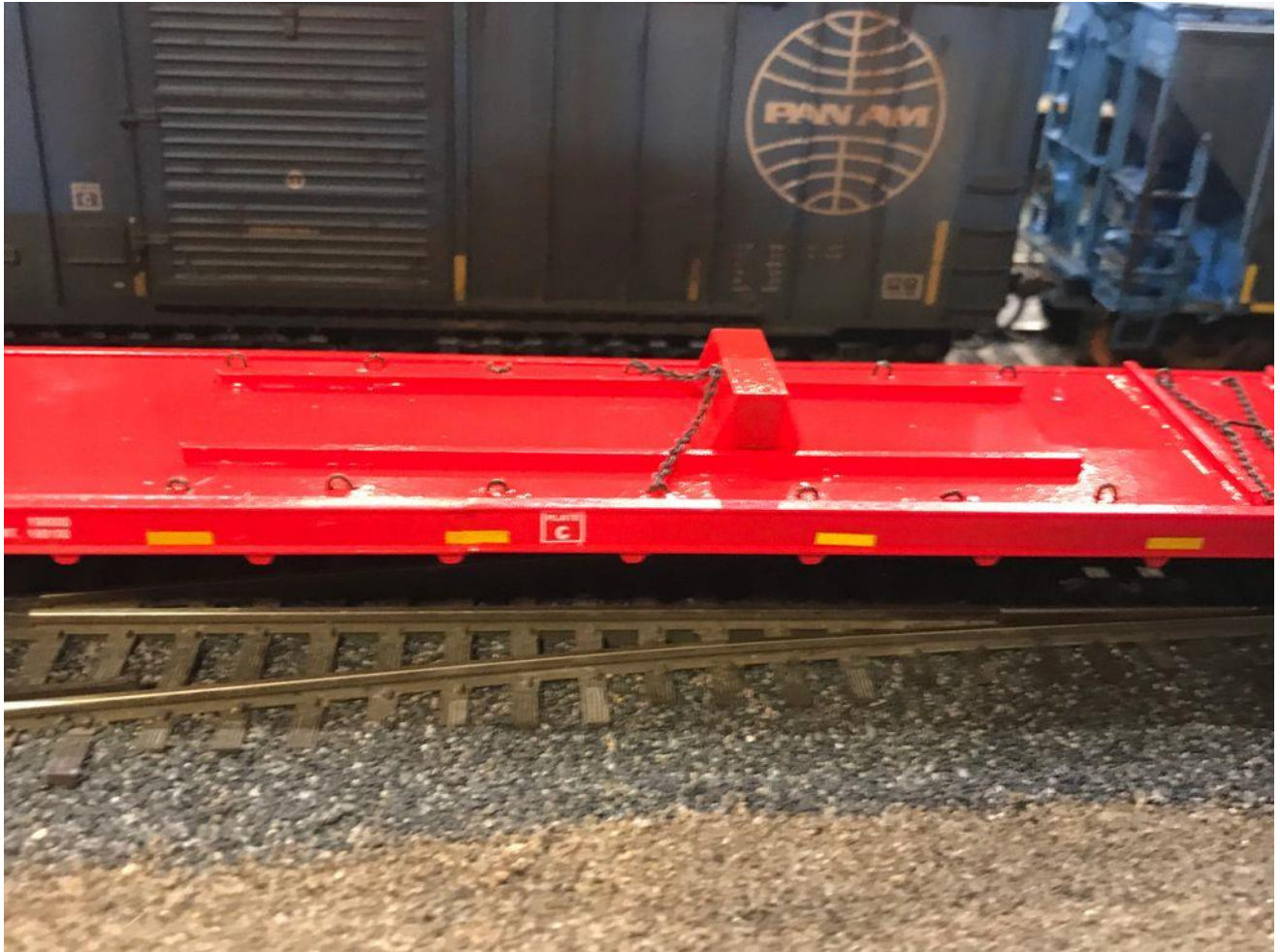
View of adjustable end showing pedestal and track system made from styrene.
