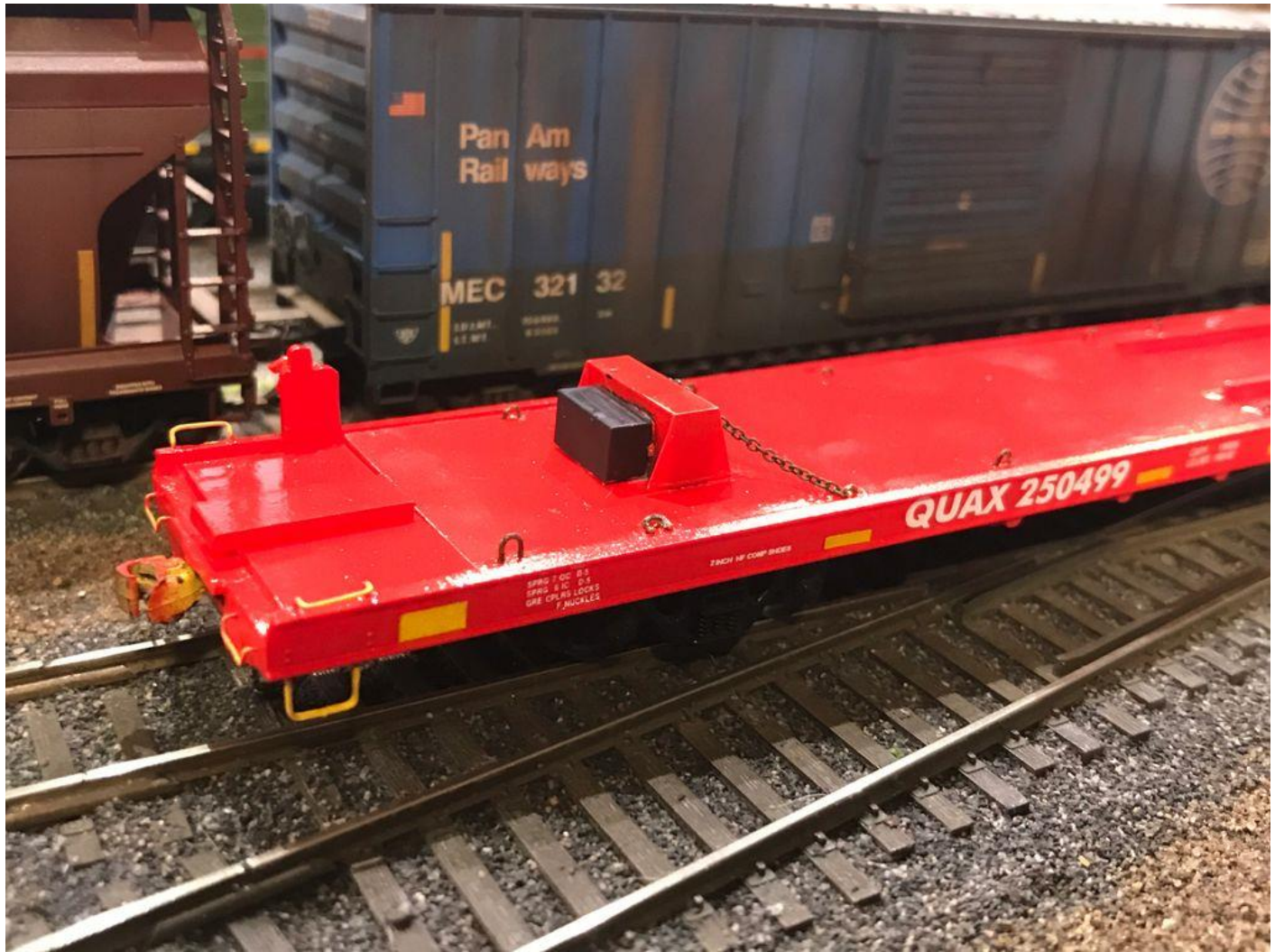
View of permanently mounted pedestal and toolbox on "B" end of car.
