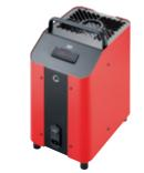
temperature calibrators of the TP Basic series. It consists of dry block calibrators which cover a wide temperature range and are used onsite e.g. in the marine sector. Designed to ensure a comfortable calibration of temperature sensors, they impress with an easy operation and a thoughtful use of different automatic functions.
