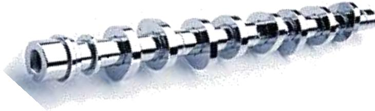
The part of engine which opens and closes the valves is called Camshaft.
