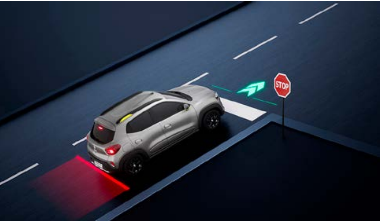
hill start assist (2) Maintains brake pressure for few seconds, preventing rollback when you move away on a steep slope.
