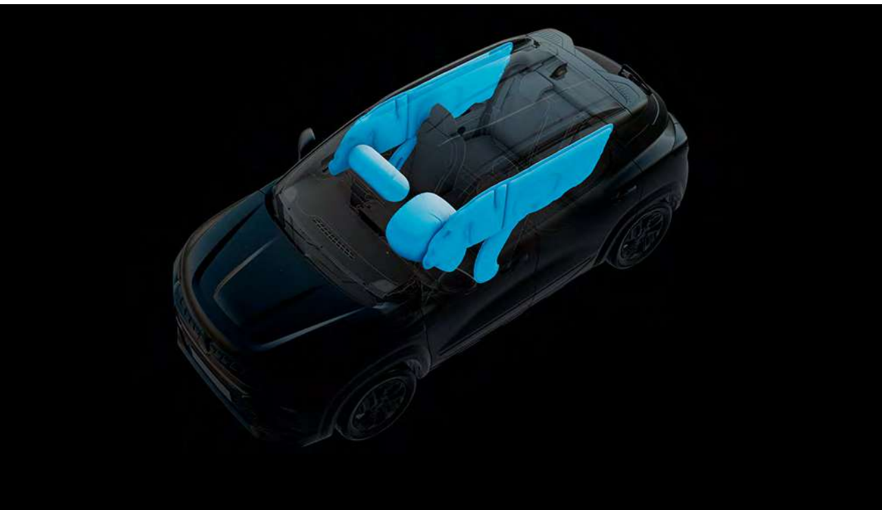
6 airbags Six airbags offer increased protection.
