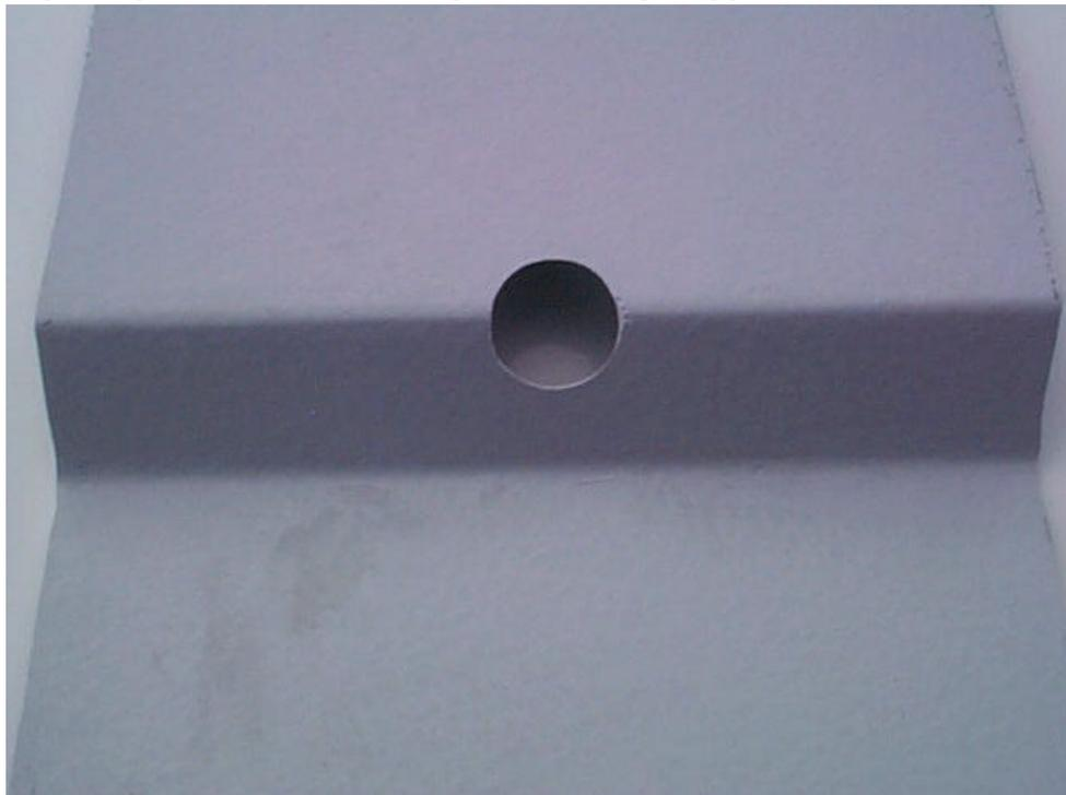
Step #1: Grind or sand the inside of the panel 3" larger than the area where the repair is required.
