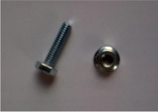
Used for bolting **end panels** internal flange together. 1/4-20 x 1" hexcap and 1/4" nut
