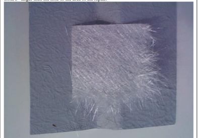
Step 4: Mix the resin required with catalyst also supplied in the repair kit. Ratio of 1 quart of resin to 1-1 1/1 bsp of catalyst. Wet the glass cloth with resin and apply to the hole or crack on the inside surface. Using a brush work out the air bubble to ensure good surface contact.
