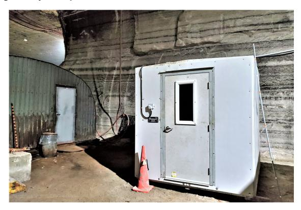
A mining company reached out to our team at RM. They needed an underground office that could be built on site in a potentially difficult location. We worked with our client to design an 8'x8' enclosure in component kit form.
