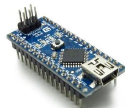
A photograph of an Arduino Nano microcontroller board. It is a blue PCB with a ATmega328P-8 bit AVR microcontroller at the center. It has a USB port for programming, a power jack, and various pins for connecting sensors and actuators. The board is oriented diagonally, showing its components and pins. | 2250 |
