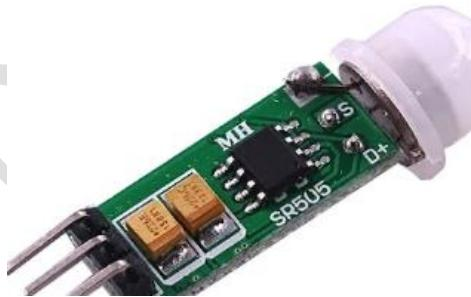
A photograph of a PIR motion detector module. It is a green printed circuit board (PCB) with a white plastic housing. The PCB has several components, including a central integrated circuit labeled 'MH', two orange capacitors, and several other resistors and connecting pads. The module is oriented diagonally, with the housing pointing towards the top right. | 2260 |
