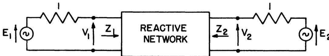
Figure I-1. Two-terminal-pair reactive network with one-ohm terminations.
