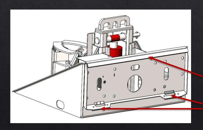
Quick attach plate has gusset on top for extra support
