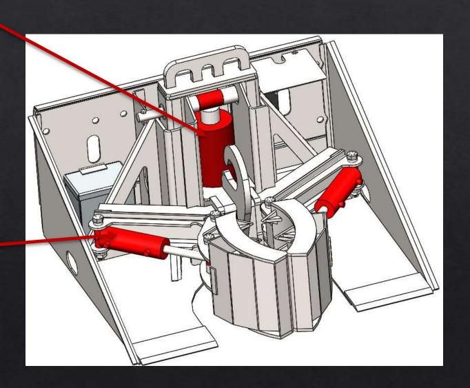
LIFTING POINT FOR PLACING POLE —
