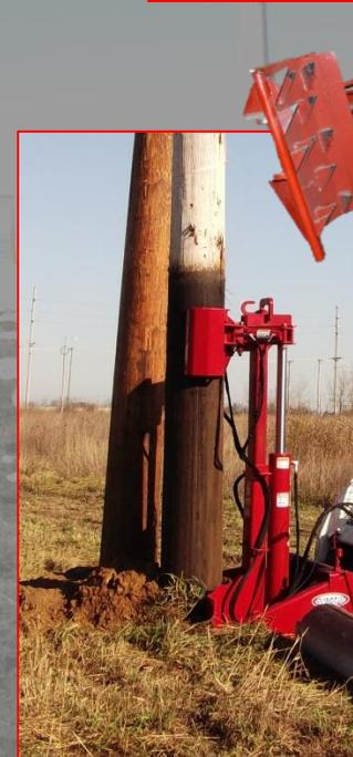
Two large 3x6 inch clamp cylinders and metal teeth on the jaws securely hold pole in place during extraction.
