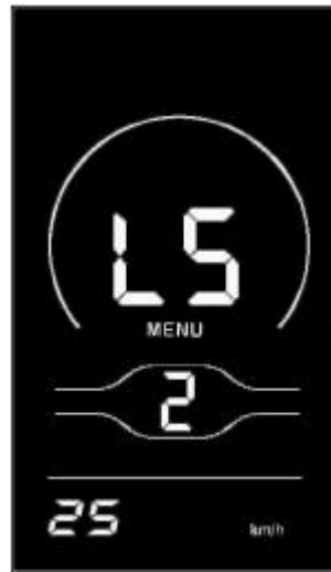
Speed limit setting interface
