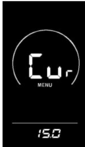
Current limit value setting interface
