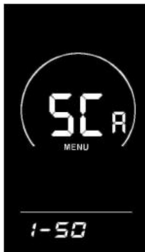
PAS ratio value setting interface
