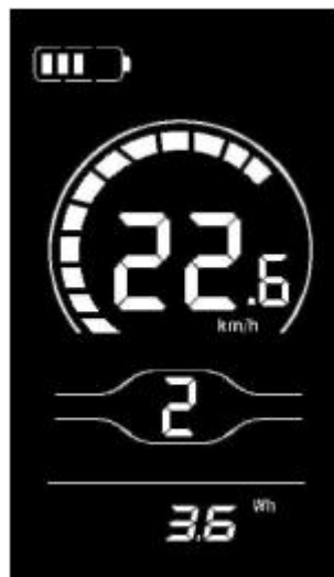
Motor power indication interface
