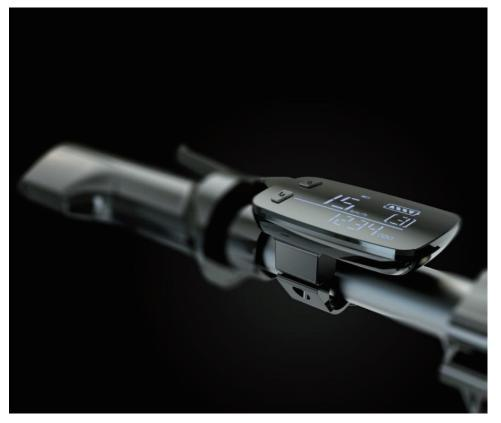
① Display: speed+unit; power indicator; mile age+unit; 3-lever assist.
