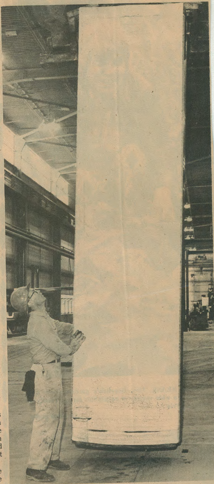
HUGE BLOCKS of aluminum, or "ingots", go into many useful products from the Troutdale reduction plant of Reynolds Metals Company. Construction, recreational, marine, household foil are just a few of the applications that come from ingot like this.
