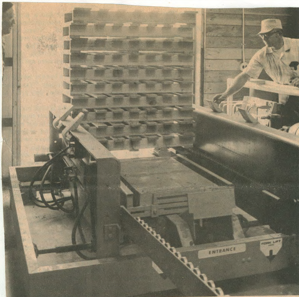
FINISHED PRODUCT. Stacker piles up pallets from the bottom. Device lifts stack and latest pallet is added from below. At
