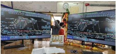
there are a total of 42 main signals, 17 independent shunt signals, and 30 dependent shunt signals. The track circuit configuration includes 67 conventional circuits and 19 axle counter MSDACs. This commissioning also involved making the middle line suitable for DN direction traffic from BPL to SUW (covering a distance of 12 km).
