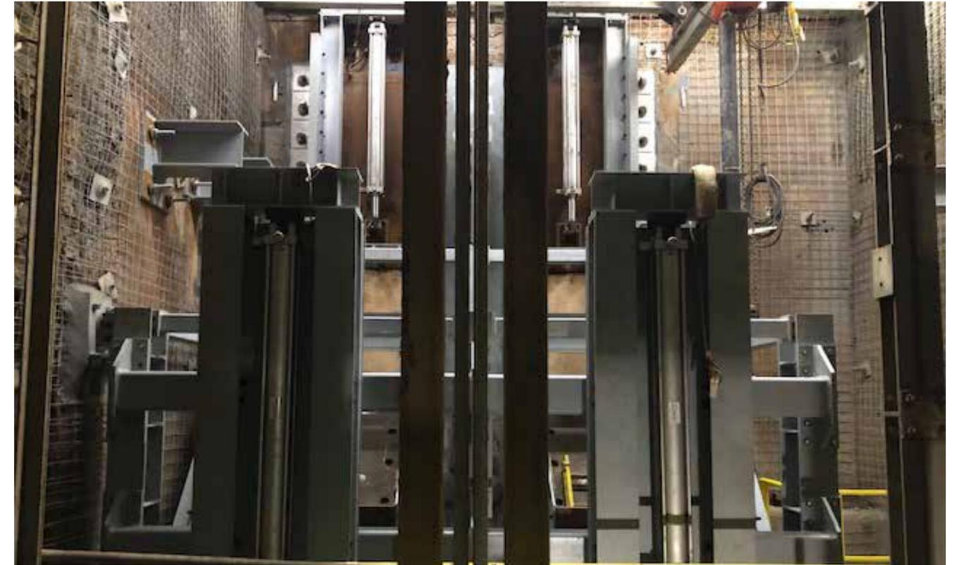
Two chutes are used to help meter and load excavated rock that will be hoisted to the surface.
