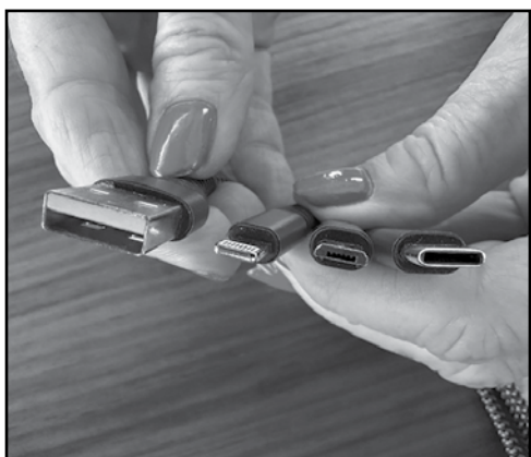
Pictured left-to-right are the standard USB (large rectangle), Apple's Lightning cable (tiny oval), micro-USB (frowning), and USB Type-C (larger oval), the latest in the evolution.
