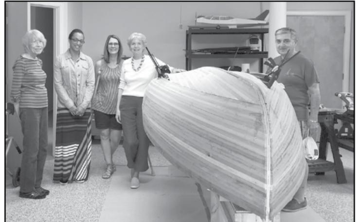
Because the boat we are building has no nails or staples, each strip has to be securely glued to the one next to it and clamped to the forms to get it to follow the hull shape. The process can't be rushed, but it gets really exciting when the hull begins taking shape and starts looking like a boat. We apply one or two strips each day on each side of the boat, so it takes about a month to complete this phase of the project.
