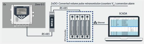
3. Process of measurement using TEC-I and turbine gas meter
