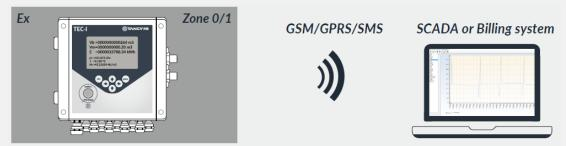
2. Remote data readout – connection through communication interfaces INT-S3, RTU controller independently
