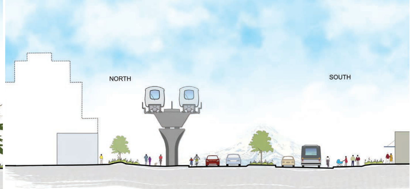
CROSS SECTION OF TYPICAL NORTH RUNNING GUIDEWAY ON FRASER HIGHWAY NEAR 152 ST
