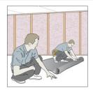
**ROLL OUT THE MLV**Roll out the MLV on the floor and mark the measurement for cutting.
