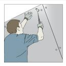
**CONTINUE FASTENING**Fasten the nail or screw with a washer 2' on center along the top and bottom plate and length of each stud.
