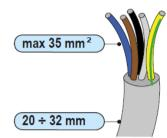
The cross-section of the AC line conductor must be sized in order to prevent unwanted disconnections of the inverter from the grid due to high impedance of the line that connects the inverter to the power supply point; In fact, if the impedance is too high, it causes an increase in the AC voltage that, on reaching the limit set by the country of installation, causes the inverter to switch off.
