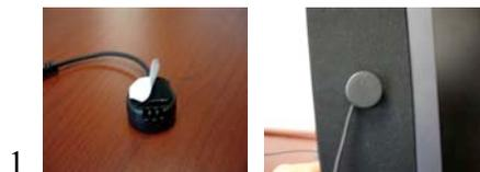
Remove the thin protective covering on the Power Microphone and stick the Power Microphone on the center of any speaker on your television. To reduce outside room noise picked up by the Power Microphone, increase TV volume.
