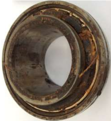
Fig.3 Lubricant: Solid, hard & dry
