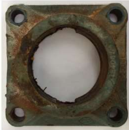
Fig.1 Housing Front: Corrosion
