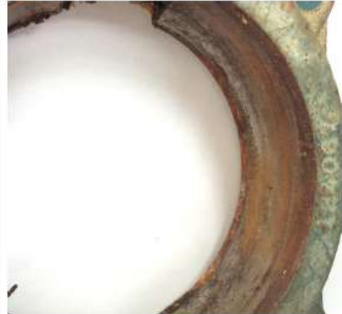
Fig.2 Housing Bore: product contamination & corrosion
