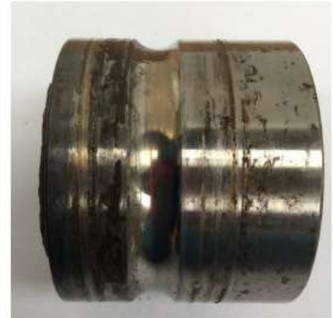
Fig.4 IR Raceway: Lubricant starv. & discolouration
