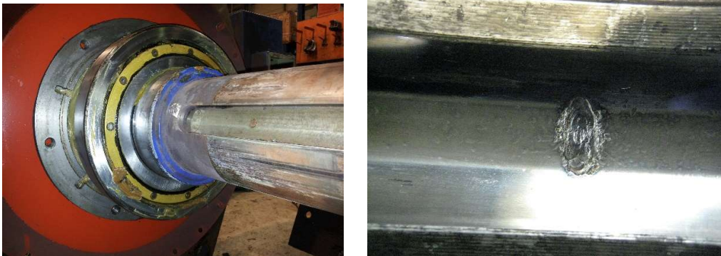
Figure 6: Drive end bearing during strip & load zone damage on outer raceway
