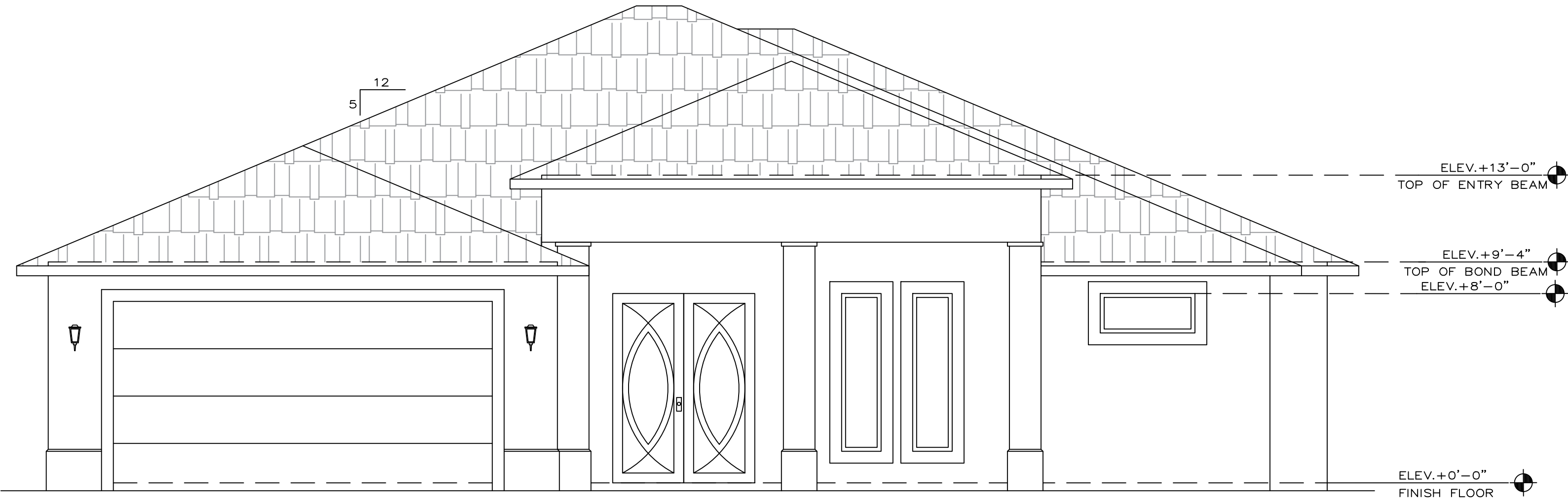
FRONT ELEVATION SCALE 1/4" = 1'-0"
