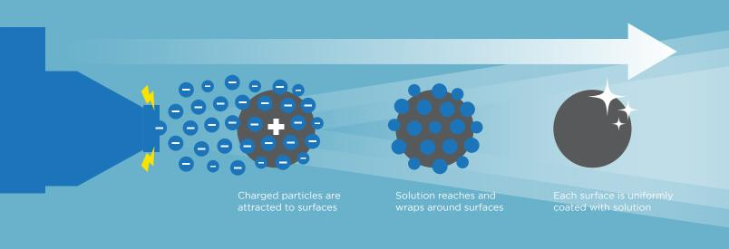
Electrostatic sprayer technology works by sending a positive electric charge through the disinfecting solution, causing it to be attracted to negatively charged surfaces like two poles of a magnet. This technology removes the liability of human error from the disinfecting process.
