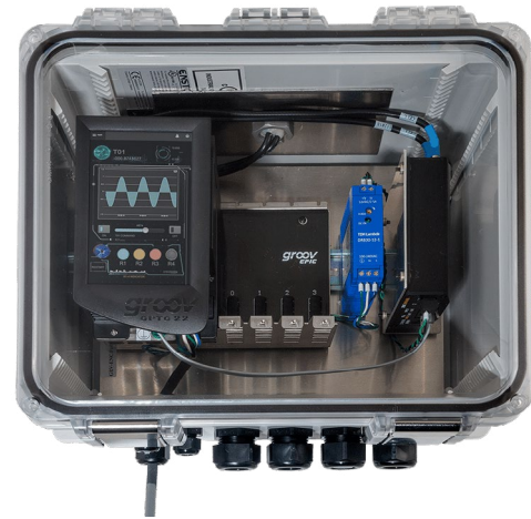
The i4.0 Accelerator, installed on an Opto 22 groov EPIC IIoT Industrial Gateway
