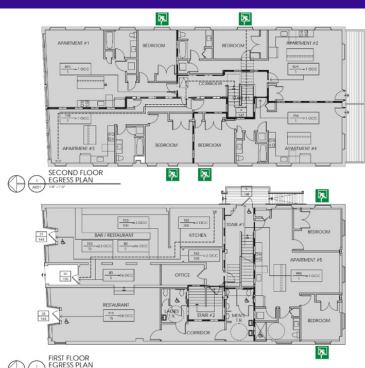
constructed in a portion of the first floor, and the entire second floor. There will be one ADA accessible (2) bedroom on the 1st floor. There will be four (1) bedrooms on the 2nd floor.
