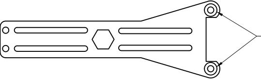
Countersunk holes for M3 Flat Head Screws when mounting directly to gearbox stay
