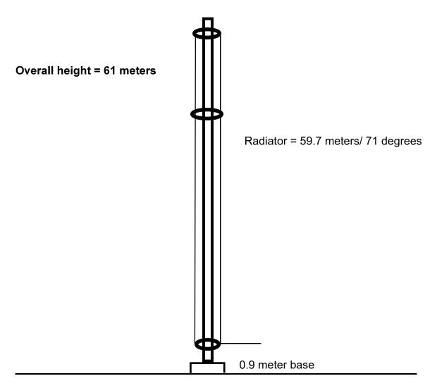
61 Meter guyed and grounded tower (59.7 m radiator) excited via a three wire folded unipole. The ground system consists of 120 buried copper radials 54.3 meters in length.
