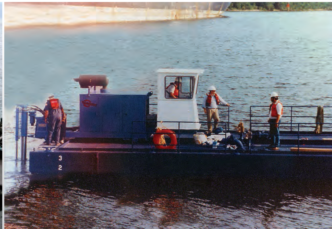
› Single Workmaster outdrive propulsion unit installed on a spill cleanup barge of MSRC (Marine Spill Response Corporation).
