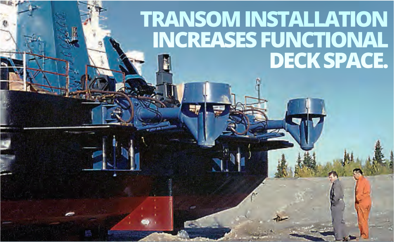
Twin transom mounted modular propulsion units with depth adjustment tilted 90°
